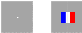
Fig. 3. Task definition: a single cell program beginning from a white state, at time 0, must replicate itself and differentiate itself into other cells, so that at iteration 6, it becomes a 63 cell French flag, and remains like that indefinitely. Initially, at the same location as the single start cell, there can be chemicals having values 0 or 255
